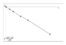
The process is of first order if the points fall to a straight line, otherwise its behaviour is different.
