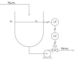
Outflow flow rate is manipulated variable, and inflow flow rate is disturbance. Process:
