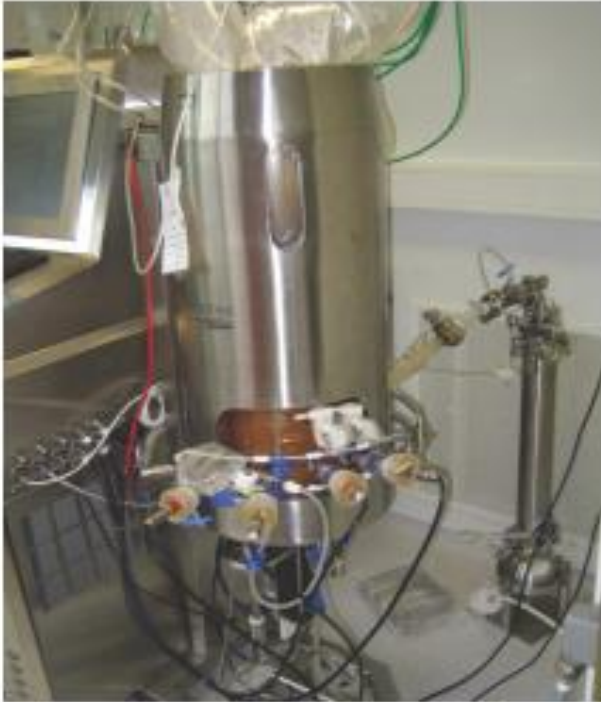
An Xcellerex bioreactor used in an intensified perfusion process with ATF System equipment ( www.refinetechnology.com )
