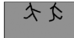
Stress corrosion cracking
