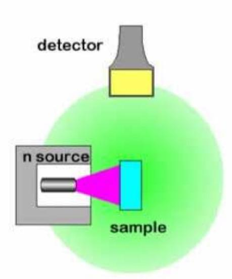
The detector must be at an off angle and shielded.
