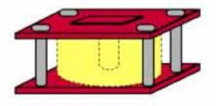
Complete mounting with lid that can and should be locked down when the source is not in use.
