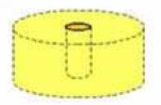
Wax mounted Pu and Be powders with a bore.
