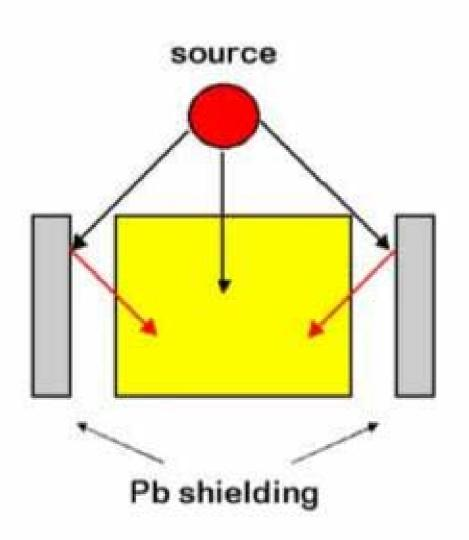
This effect can be reduced by moving the shielding farther away from the detector/source
