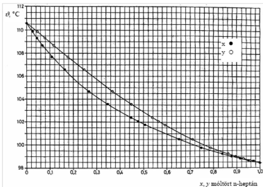
Fig 4. Bubble point – cloud point diagram of n-heptane - toluene
