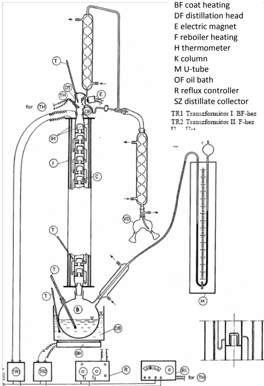
Fig 3. The laboratory batch rectification column
