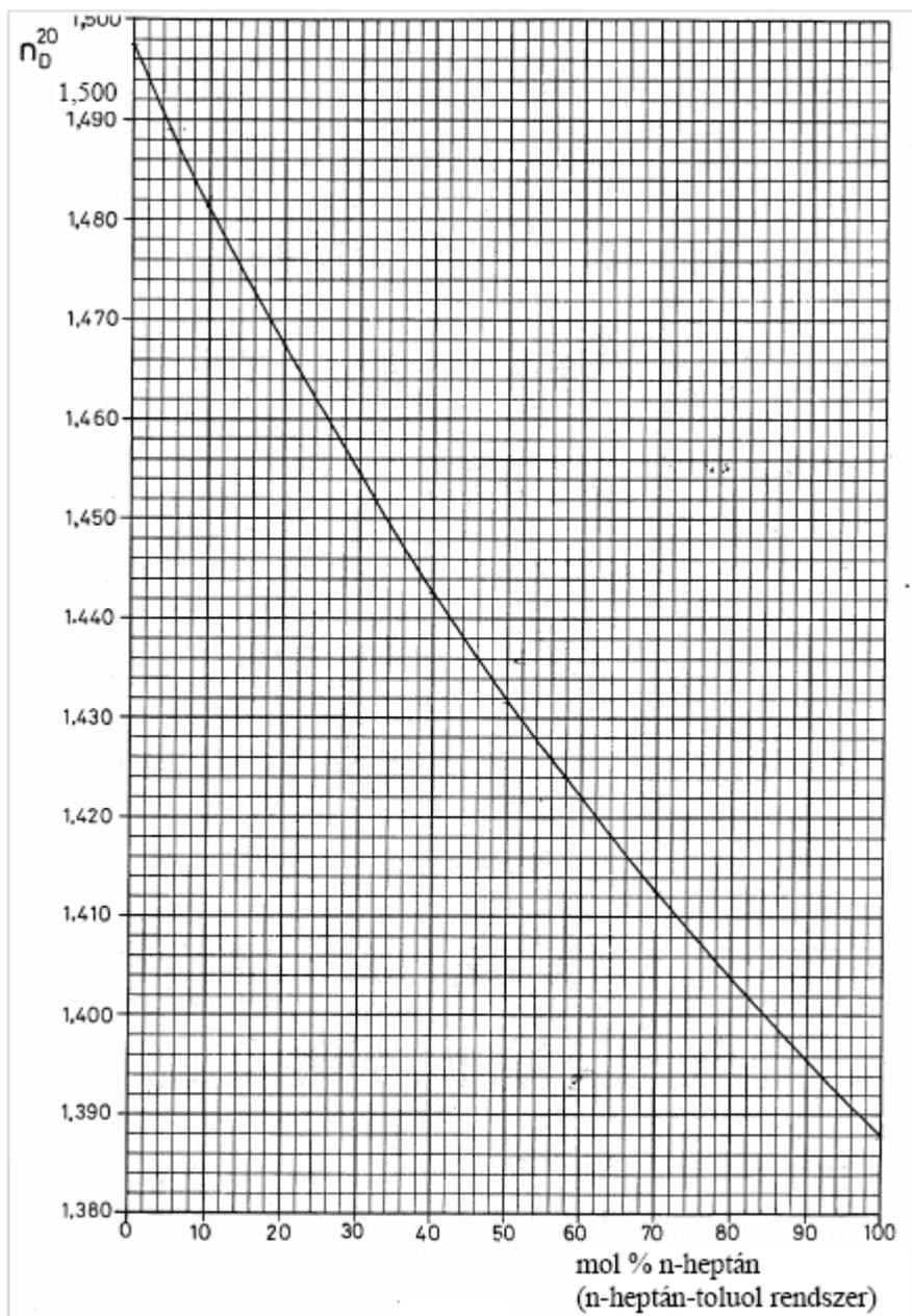
Fig 6. Refractive index – composition calibration diagram
