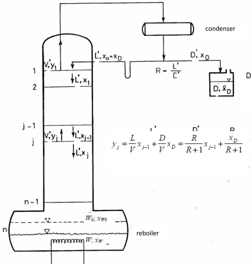
Fig 1. Schematic representation of a batch rectification unit
