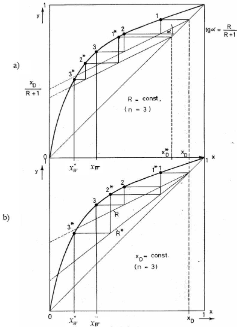
Fig 2. Two basic ways of operation a batch rectification unit
